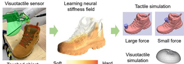
Fig. 1. Our method estimates a high-resolution stiffness field of a deformable object using a visuotactile sensor. The estimated stiffness field can simulate contact forces for novel touches and the deformation of the visuotactile sensor upon contact with the object.
