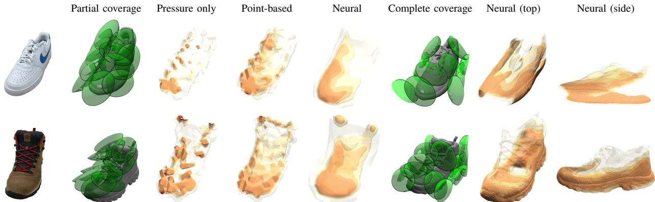
Fig. 2. Qualitative stiffness estimation comparison of Pressure-only, Point-based VSF, and Neural VSF using dense force estimation. Following partial coverage, the left columns show the estimated stiffness using top-down touches on the object. The right two columns demonstrate improved Neural VSF estimation with an SDF mask and multiple touches from different directions for complete coverage.
