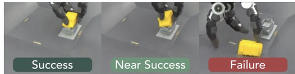
Fig. 3: **Experimental outcomes.** We consider three outcomes for the plug insertion trials: success (left), near success (middle), and failure (right).
