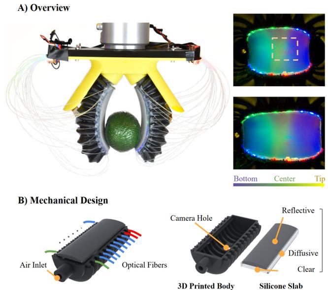
Fig. 1. (A) Overview of the proposed soft robotic tactile and proprioceptive system. (B) Mechanical design of the PneuGelSight sensor.
