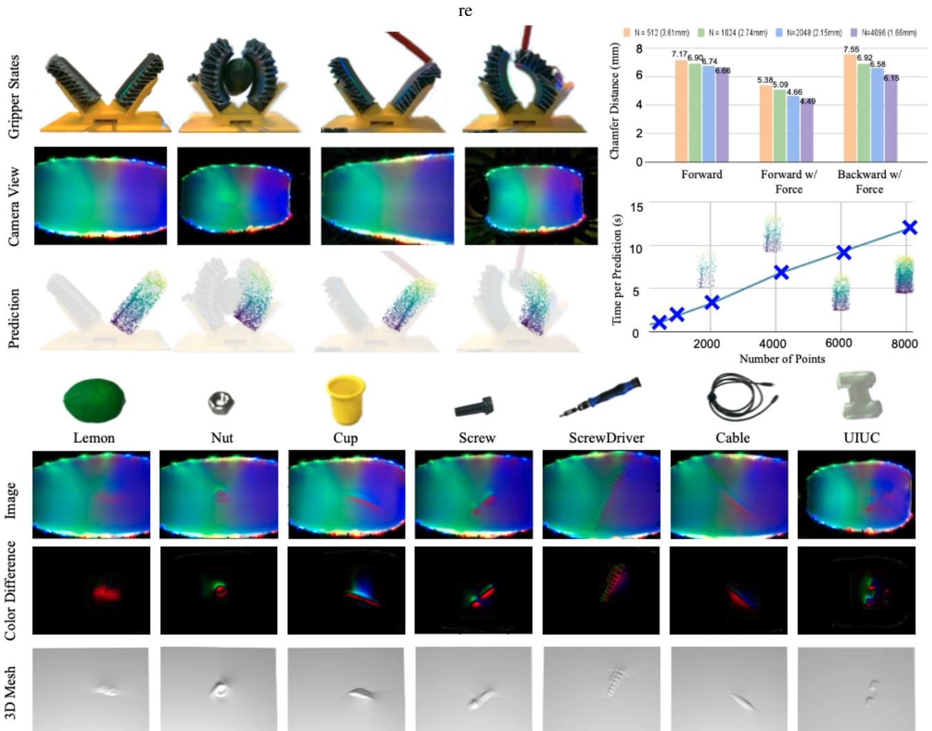
Fig. 2. Accuracy of proprioception and tactile sensing. We analyze the impact of sampled point cloud intensity on proprioception accuracy (top right) and qualitatively assess the sensor’s texture reconstruction capability (bottom row)
