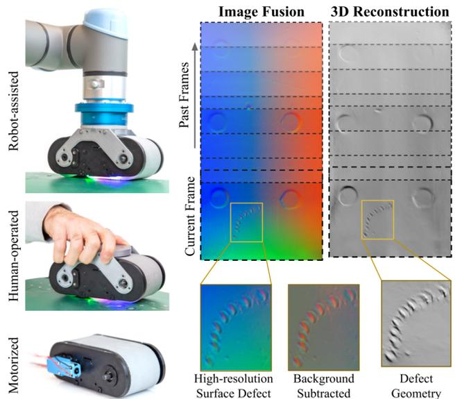
Fig. 1. The GelBelt sensor can be mounted on a UR5e robotic arm, operated by a human, or motorized to scan large surfaces.
