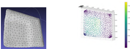
Fig. 3: For the rectangle example: (left) illustration of the deformation; (right) stress applied on it.
