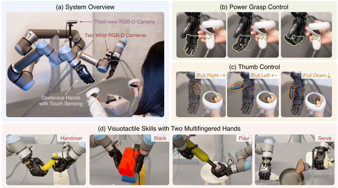
Fig. 1. An overview of our system setup and learned visuotactile skills on four tasks. (a) Our hardware and teleoperation system setup. The hardware consists of two UR5e robot arms, each equipped with a Psyonic Ability Hand. Visual observations are obtained via two wrist RGB-D cameras and one third-view RGB-D camera. Tactile observations come from the multifingered hands, with each fingertip equipped with six touch sensors. We utilize the Meta Quest 2 platform for teleoperation. (b) We use grip buttons of the Quest controllers to command power grasp of the non-thumb fingers. (c) We use thumbsticks to control the 2-DoF joint positions of the thumbs. (d) Four policies learned from visuotactile data collected by our hands-arms teleoperation system (HATO). These policies can accomplish a variety of complex bimanual tasks: handing over slippery object, stacking block tower, pouring from a wine bottle, and serving steak.
