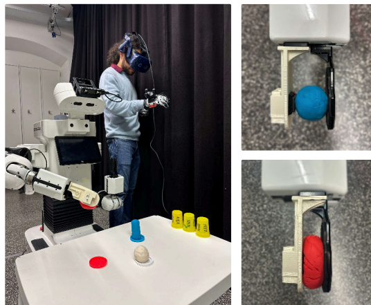
Fig. 1: The Teleoperation setup. Left - Tiago Robot equipped with tactile GelSight sensor. Right - Comparison of soft and hard grasps of modeling compound.
