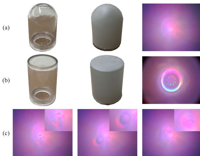
Fig. 2. (a) and (b) represent RoTip sensor with a hemisphere tip and a flat tip , respectively. The first two rows display, from left to right, the transparent support shells, the coated elastomer, and the tactile images. Sparking points are noticeable due to the intense reflection from the flat tip. (c) displays the tactile readings captured as the hemisphere-tipped RoTip sensor interacts with a bolt, a nut, and a USB cable.
