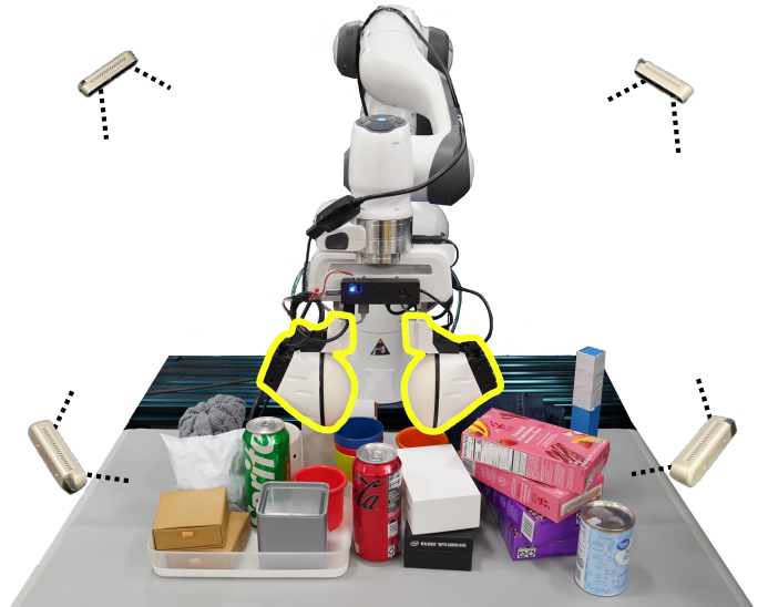
Fig. 4: Hardware overview. Our experimental platform consists of a Franka Panda arm, two Soft-Bubble grippers, four RealSense D415 RGBD cameras, and a diverse set of objects.
