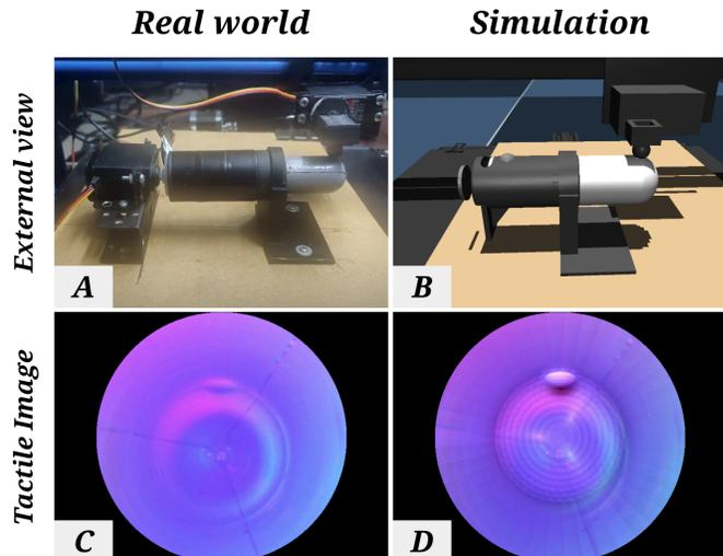
Fig. 1. (A) and (B): The real and the simulated experimental setups respectively, in each a GelTip tactile sensor is mounted onto a 3D Printer and contacts a 3D printed object (here is a cube with a hollow cylinder in the centre). (C) and (D): The corresponding tactile images captured from the GelTip sensor, real and simulated respectively.
