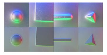
Fig. 2. **Real vs. virtual tactile images.** Samples captured by a real GelSight sensor (top) and generated virtual correspondences using our method (bottom).
