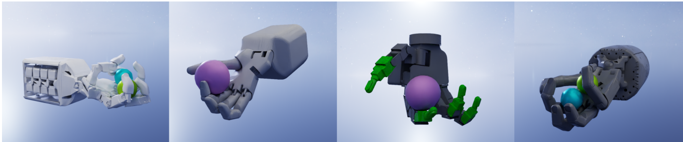
Fig. 1. The roto 2.0 Benchmark Suite : A standardised RL framework across four distinct dexterous morphologies (from L to R): ORCA Hand, Shadow Lite, Allegro Hand, and the Shadow Dexterous Hand. The suite facilitates “blind” tactile manipulation tasks, such as Baoding ball rotation and ball bouncing.
